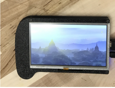
Figure 2: Touch screen device for the clinician. The black casing is designed to hold easily with one hand.
