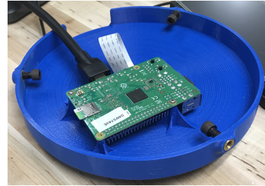
(b) Raspberry Pi is securely fastened to housing by 3 small screws.
